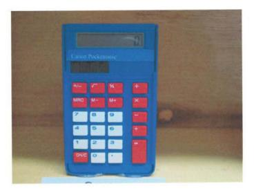
THE CANON POCKETRONIC WAS THE FIRST HAND HELD CALCULATOR. IT WAS MANUFACTURED IN JAPAN IN THE MID-1971. WHEN IT BECAME AVAILABLE, IT COSTED ABOUT \$395. IT WEIGHED ABOUT 1.8 POUNDS, AND WAS 4 INCHES WIDE, 8 INCHES LONG, AND 2 INCHES HIGH. IT WAS A FOUR FUNCTIONED CALCULATOR WITH A CAPACITY OF 12 DECIMAL DIGITS.
