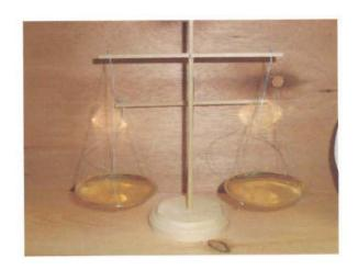
WEIGHING PLAYED AN IMPORTANT PART IN THE ANCIENT EGYPTIAN'S LIFE. THE BALANCES EMPLOYED WERE ORIGINALLY OF SIMPLE PATTERNS AND EXISTED BEFORE 3200 B.C. THEY CONSISTED OF TWO COPPER AND SILVER PANS SUSPENDED BY CORDS AT THE ENDS OF A CENTRALLY SUPPORTED HORIZONTAL BEAM. IT MAIN PURPOSE WAS TO WEIGH METAL.
